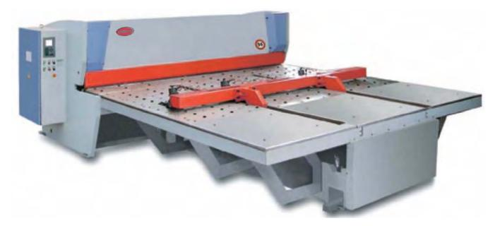
The LSGK series is also available in front-feeding models with thickness capacities of  $\frac{1}{4}$ " and  $\frac{5}{16}$ ", and lengths of 10 feet or 12 feet.
