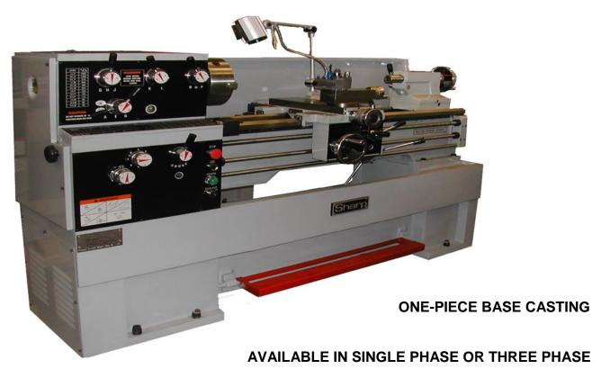
The SHARP SH1440 lathe is exceptionally heavy and rigid for its size. The bedway width is 10<sup>1</sup>/<sub>2</sub>". These machines feature a 1 9/16"spindle bore. **The base casting is one piece - from end to end**. The bedways and headstock gears are precision hardened and ground and the fully enclosed quick change gearbox allows a full range of inch and metric threading. A clutch overload system protects the apron feeds.
