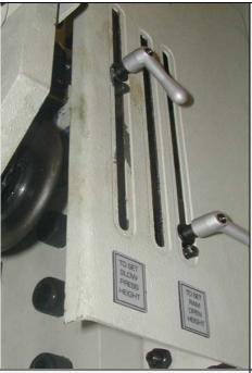
Ram open height and height at which fast ram approach changes to slow pressing speed are easily adjustable.
