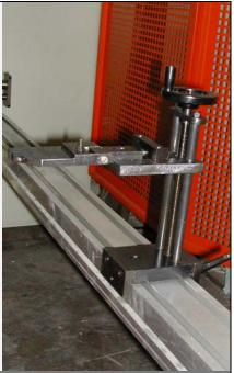
Height-adjustable back gauge fingers are clamped to a heavy wall ribbed aluminum fence.
