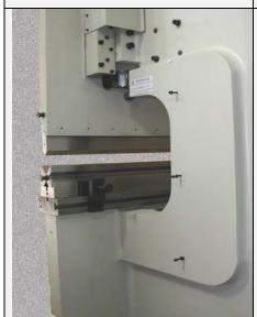
Deep throat areas are reinforced by double thickness side frames to prevent distortion.
