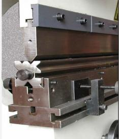
North American style tooling, slotted riser block and wide bottom table allow for a wide range of tooling set-ups.
