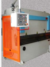
Electrically interlocked, hinged guarding prevents entry into dangerous locations during bending.
