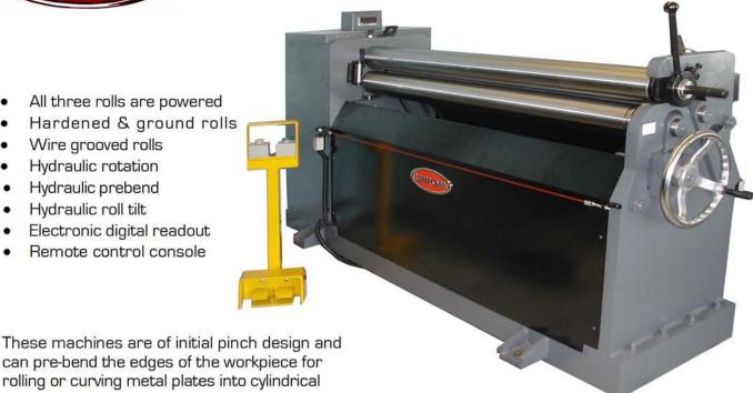
forms. The hydraulic pre-bend can provide a nearly perfect circle by reversing the workpiece after prebending. The top roll swings open to allow removal of the finished workpiece.
